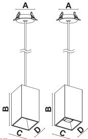
Suitable for Ceiling thickness 5-20mm.
